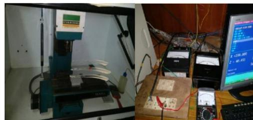
Fig.6 CNC Milling machine power measurement.
