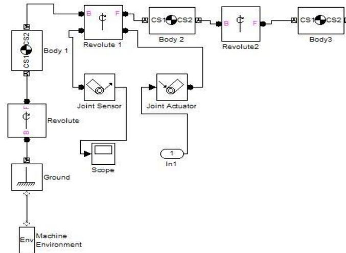
**Figure 5: Model of three links (SimMechanics toolbox)**
