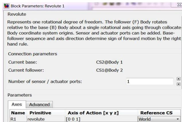
**Figure 8: revolute joint block parameter**
