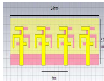
Fig.8 Layout Design of Four Elements Phased Array
