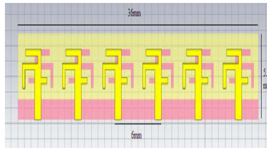
Fig.11. Layout Design of Six Elements Phased Array
